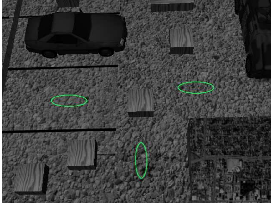
Figure 4.14: Sample camera image of landing site showing three general safe landing areas.
